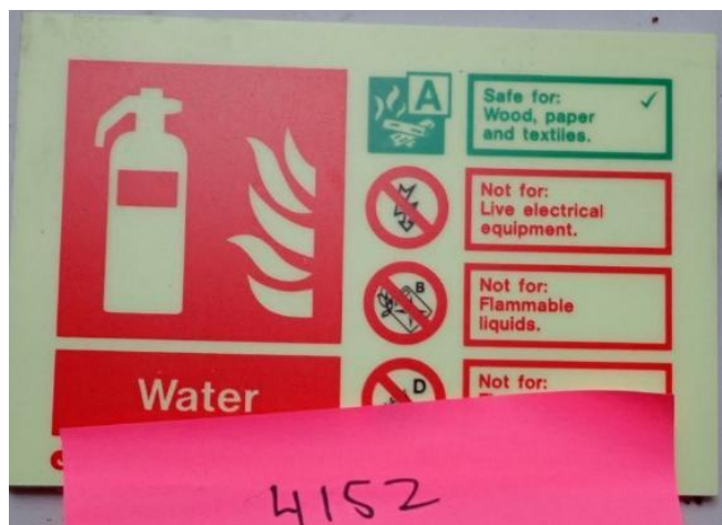
Photograph 4.3 Sample 4152 fire signage containing elevated SCCPs
