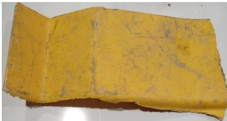
Photograph 4.2 Sample 1080 plastic casing – bromine 113,000 mg/kg
